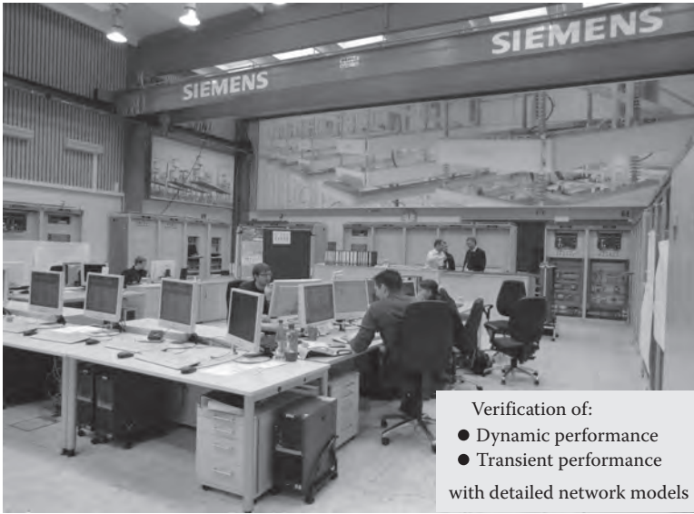
FIGURE 5.41 Example of HVDC/FACTS off-site testing in a real-time digital simulator.
